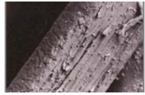
Severely Damaged: Bonds are weak and/or broken
